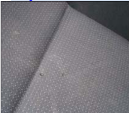
Brandgat in de stoelbekleding
